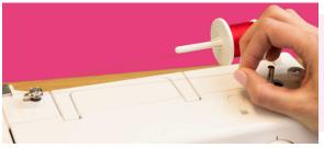
• Place thread on spool pin with the thread coming from the underneath following the numbered thread path to the bobbin winder making sure that the thread is seated firmly in the bobbin winding thread guide
