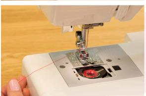
• Bring up the bobbin thread by holding the needle thread and turning the handwheel counterclockwise. The bobbin thread will loop around the needle thread. Pull the loop through to retrieve the bobbin thread.
