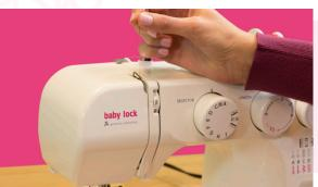
Raise the presser foot. Turn the handwheel counterclockwise to bring the needle up to the highest position so that the take-up lever can be threaded (step #3 on the machine). Finish threading through the last thread guides.
