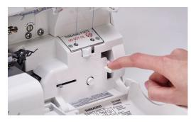
Jet-Air™ Threading With just the touch of a lever, thread is sent through the tubular loopers. There are no thread guides, no struggling and there's plenty of time to serge away.
