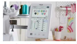
New Thread Spool Diagram on Screen The thread spool indicator diagram shows which spools need to be changed or threaded for a design. They also alert you to which spools need attention if an error such as a thread breakage occurs.
